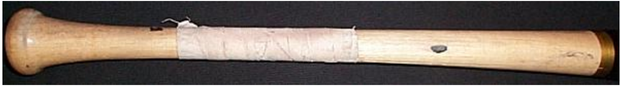
Photo A: A grain slope test spot is located 12.5" up from the knob end on the top edge grain. White athletic tape is wrapped around the crack.
