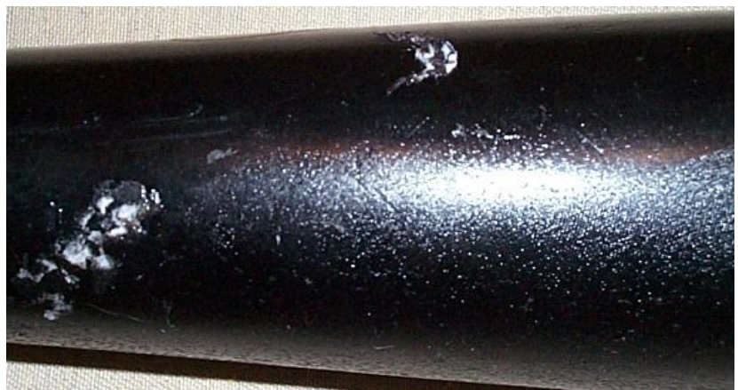
Photo G: White residue and rough texture on barrel.
