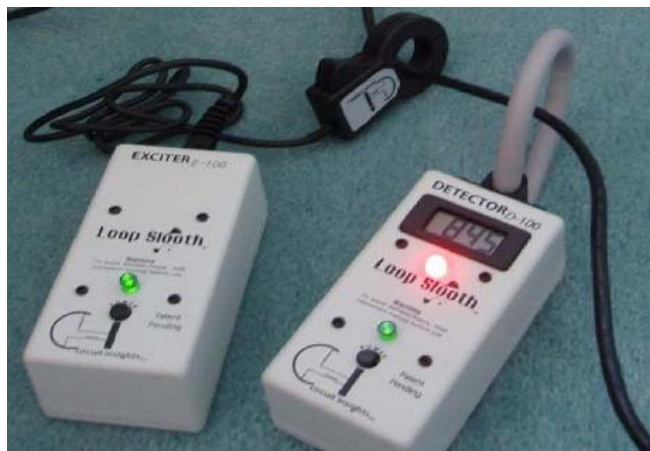
Detector indicating current driven in ground loop by Exciter (cable linked by both Exciter and Detector is part of ground loop)
