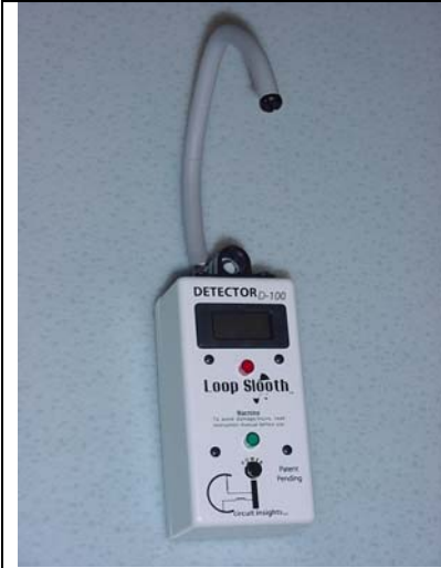
Figure 5 Detector module with its Rogowski coil open.
