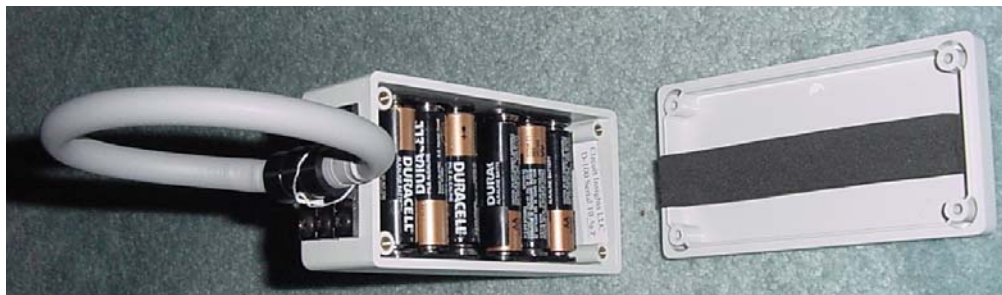
Figure 10 Back cover removed to show batteries (six AA batteries per module).
