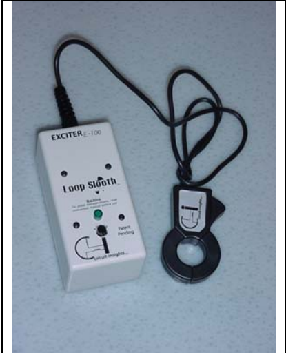
Figure 4 Exciter module with its clamp-on current transformer.
