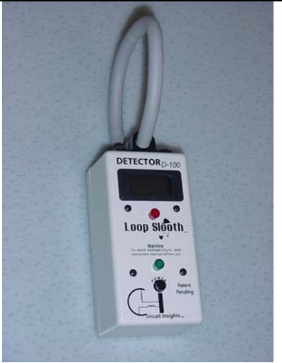
Figure 6 Detector module with its Rogowski coil closed.
