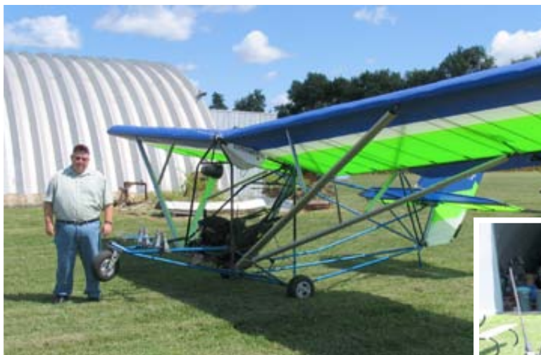
N2663R (Pixie Girl) Joe Kalal and Keith Smith's Sky Raider with Rotax 503 Engine, stationed at Gateway Air Park. (Right)
