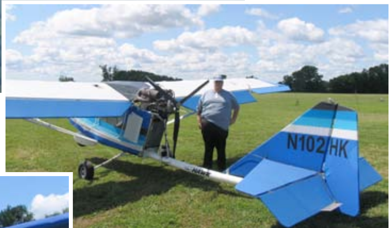
N56215 Al Bane's Quicksilver Sport 2S with a Rotax 582 engine. Stationed at Litchfield Airport. (Left)
