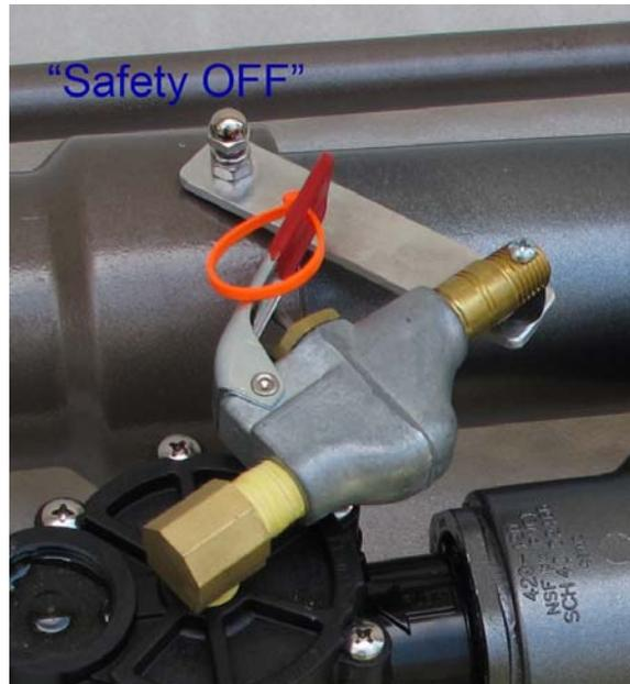
**Trigger "Safety OFF" – Trigger is released and ready**
