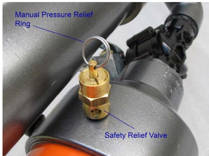
**Safety Relief Valve will open automatically if pressure exceeds ~ 90 PSI
