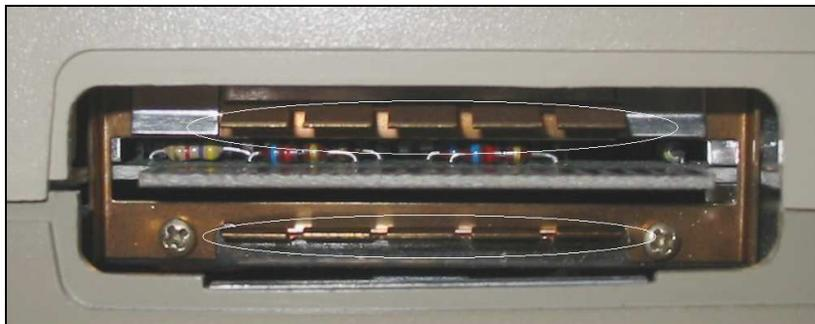
**Figure 3 - Copper Bushings**
